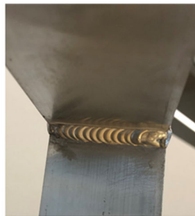
1-6: TIG welding to quality level 'C'
