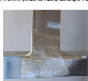
7-8: Surface grinded for smooth mounting of twin wall
